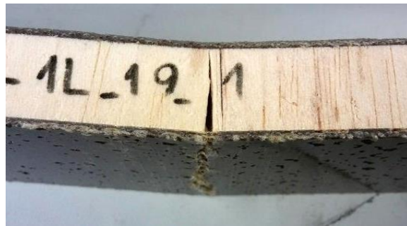
Pure core failure: vertical core break under the application point of the load. The crack goes from the bottom until the top skin layer
