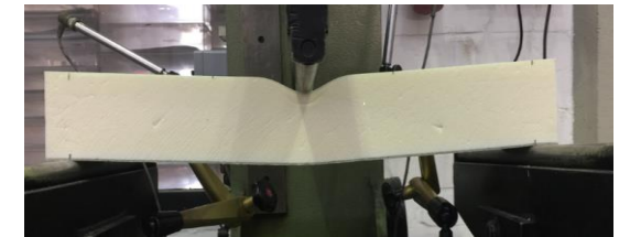
Indentation failure: 4-layer FFRP (top) and 2-layer GFRP (bottom) skinned 80 mm XPS panel
