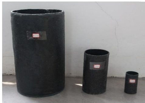
FFRP tubes: large (300 x 600), medium (150 x 300) and small (75 x 150): unit of mm
