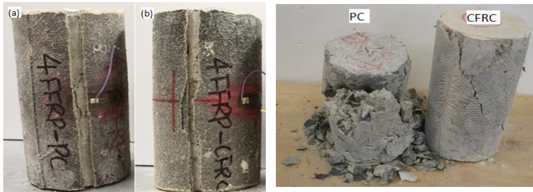
Plain concrete (PC) and CFRC cores after removed FFRP tubes
